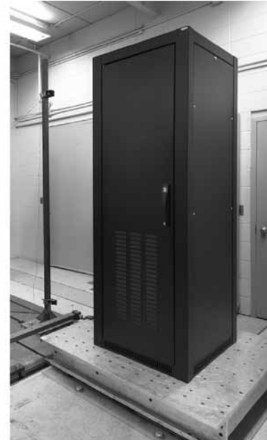
Enclosure mounted on shaker table
